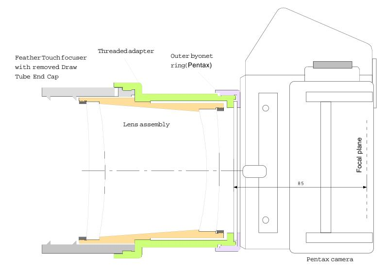
The distance from FF's base plane to the focal plane is 85mm, holding this distance is more critical for Pentax 6x7 and 35 mm cameras and less critical for CCD cameras with small chip size.
