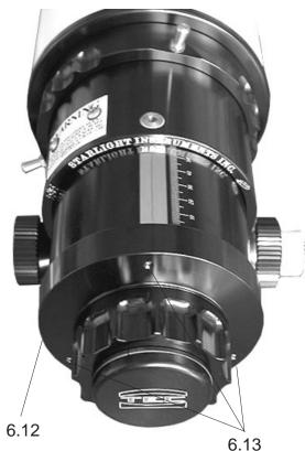
be removed. To do so first loosen all three Draw Tube End Cap Locking Screws (6.13) with 1/16" hex key and then unscrew the End Cap. Thread the Field Flattener onto the focuser drawtube to the end of thread, but do not overtighten it.
